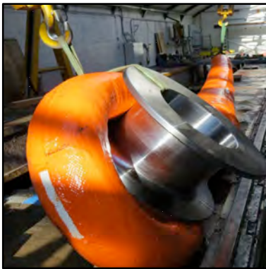
Full Size Mooring Polyester Thimble Insertion for Testing
