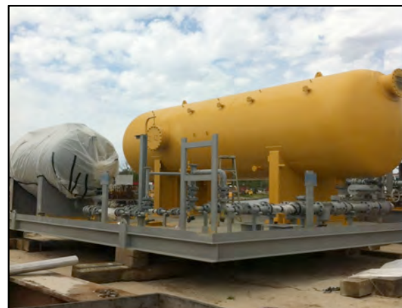
HP/LP Flare Scrubber Skid
