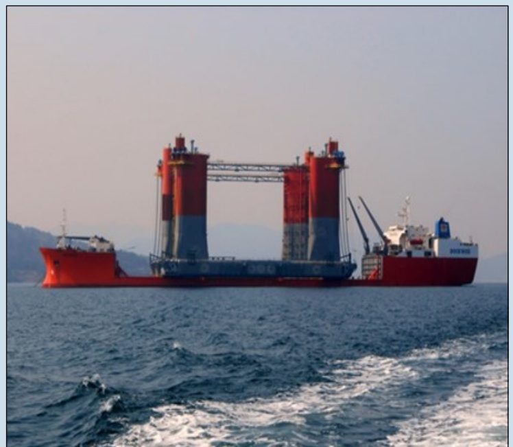
Hull Load-out onto Dockwise Vessel
