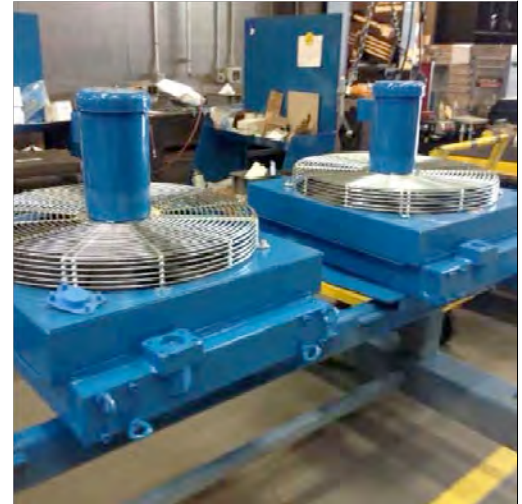
Mooring Jacking System HPU Heat Exchangers
