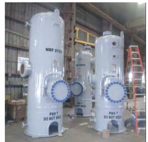
Suction/Discharge Scrubbers— Ready for Shipment
