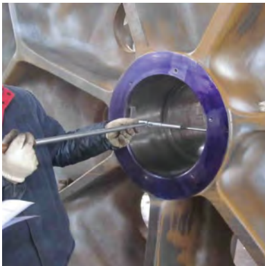
Mooring Fairlead Wheel— DNV Dimensional Verification (all found to be within tolerance)
