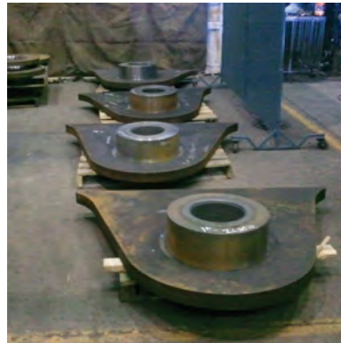
Mooring Fairlead Wheel— DNV Dimensional Verification (all found to be within tolerance)
