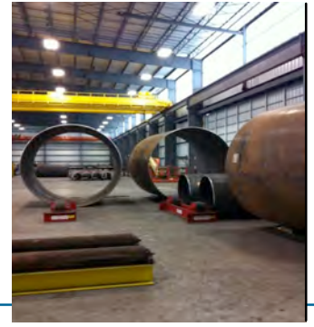
Treater 2 rolled awaiting fit up of girth seams 120"x30'
