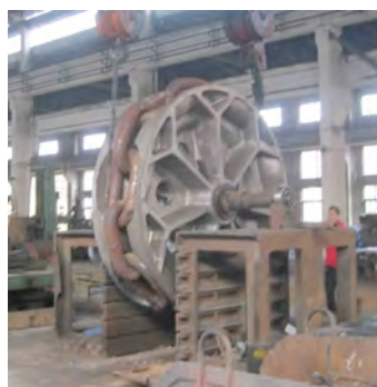
Mooring Fairlead Wheel— Chain Wrap Test
