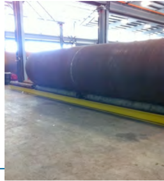
Degasser 1 completely rolled and welded 72"x20'
