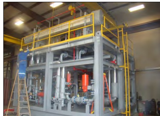
Fuel Gas Skid
