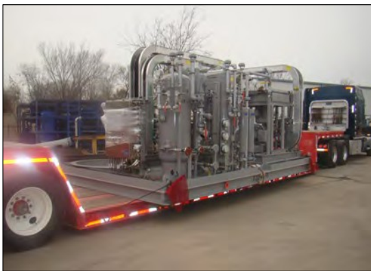
Instrument Air Skid
