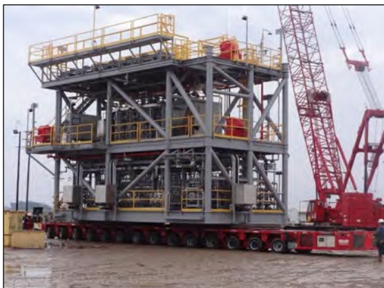
Chemical Injection Module
