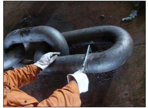
Mooring Pre-production Chain Dimensional Checking
