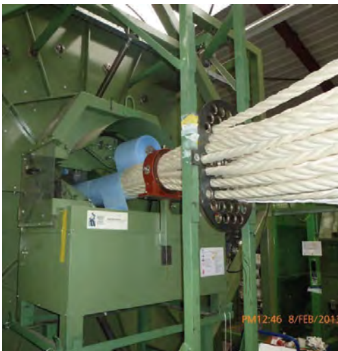
Mooring Sub ropes and Sand Filter Assembly
