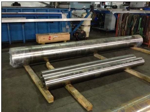
6" and 16" Pipe for Stress Joints
