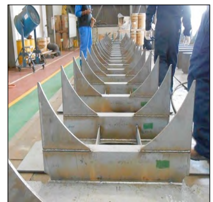
Pontoon Tunnel Section
