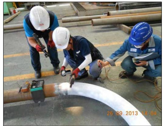
Riser Pipe Production Bend Test
